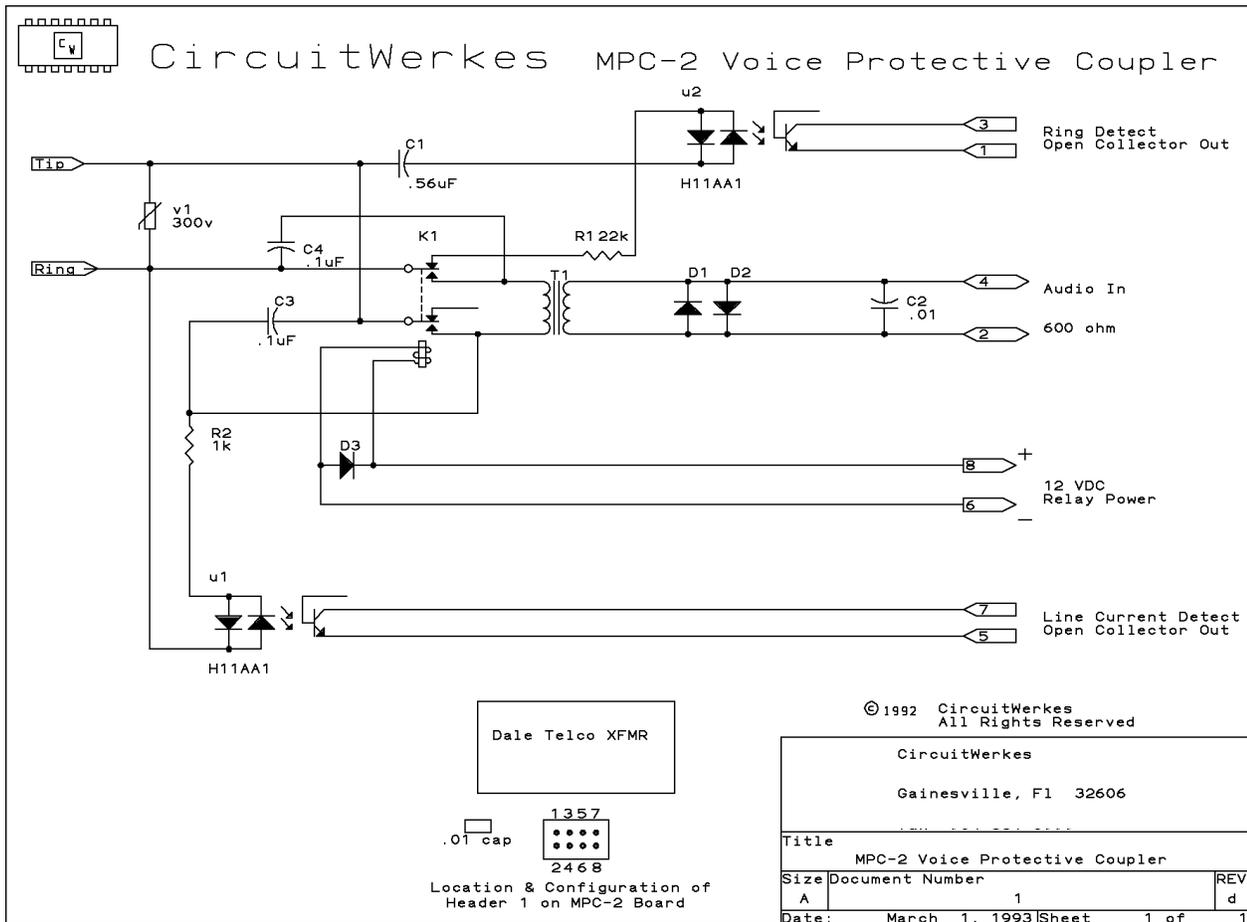
Figure 1. The MPC-2's Schematic diagram.
